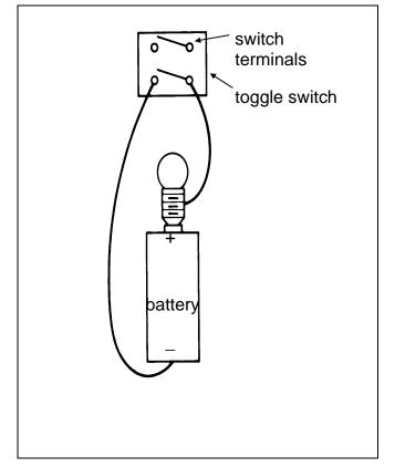
Figure B-1. Toggle Switch Continuity Test.
